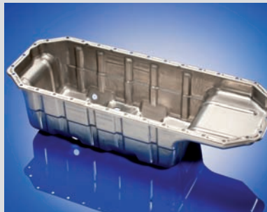
Oil pan off-highway vehicles 932 x 345 x 250 mm | DC06 t=2.0 mm
