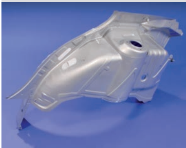
Resistance spot welding | wheelhouse assemblies 1000 x 400 x 400 mm
